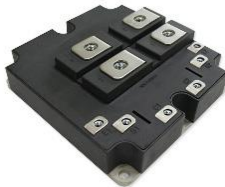
Hybrid SiC power module
