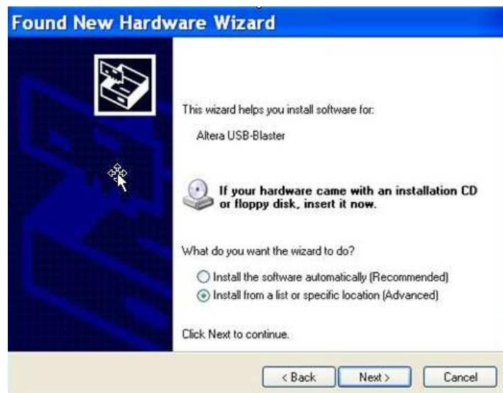
**Figure 1-3 The driver is found in a specific location**
