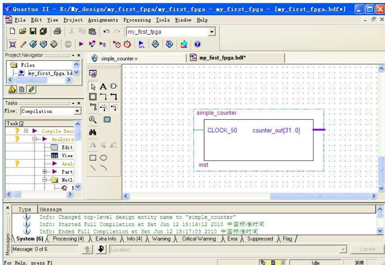
**Figure 3-7 Placing the simple\_counter symbol**
