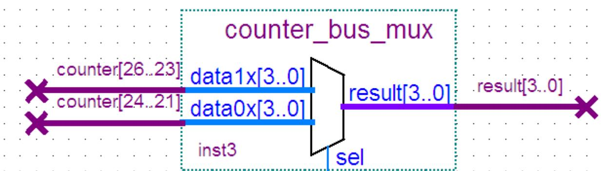
**Figure 3-26 Renamed counter\_bus\_mux Bus Lines**
