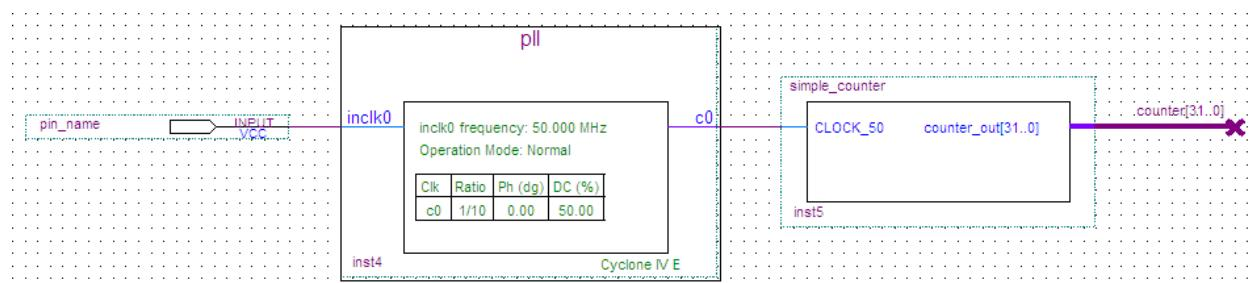
Figure 3-18 Connecting the PLL symbol and Input port
