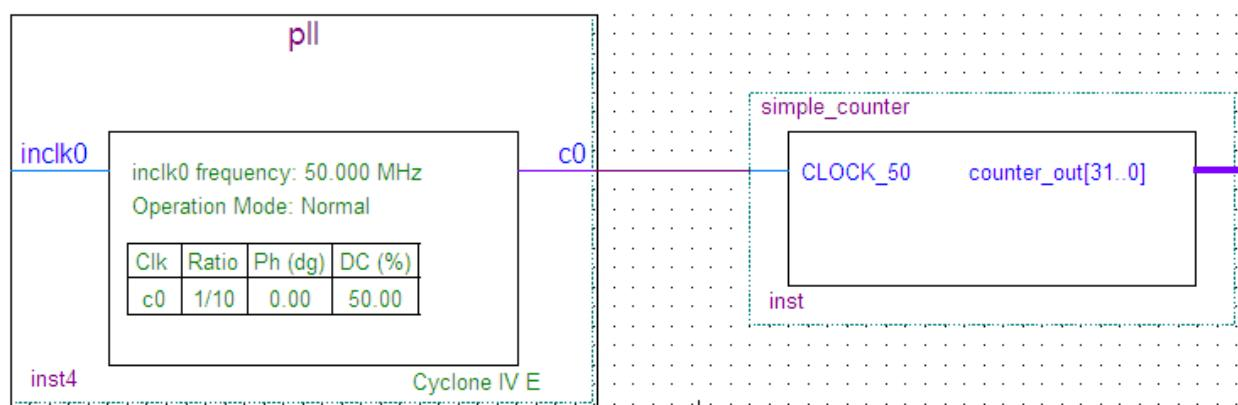
**Figure 3-16 Draw a Bus Line connect pll c0 port to simple\_counter CLOCK\_50 port**
