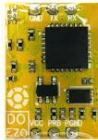
Fig. 6. Atlas EO Dissolved Oxygen Kit
